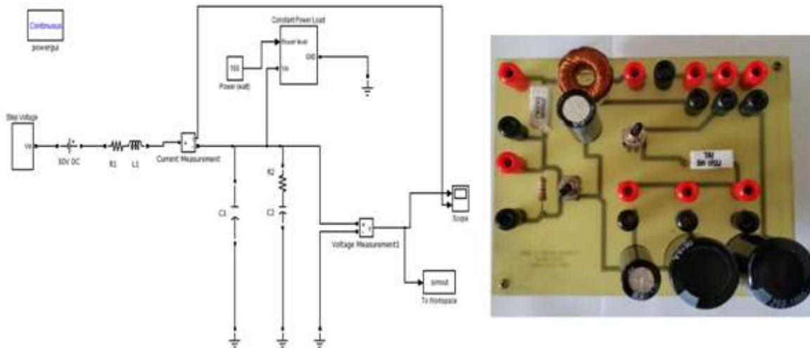
Figure 5. DC system model with RC parallel passive damping Figure 6. Hardware circuit implementation
