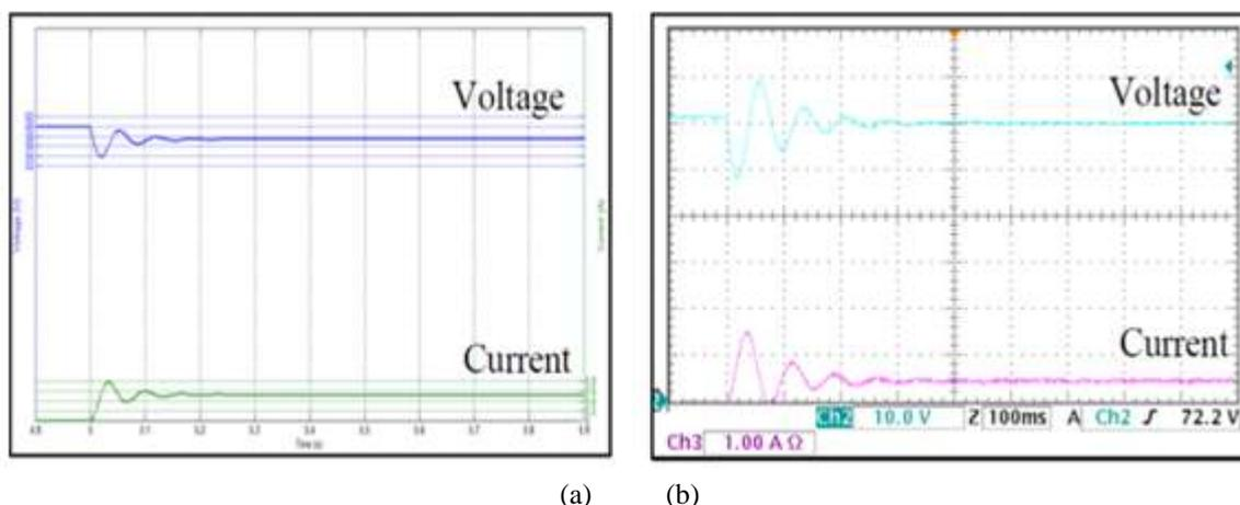
Figure 9. Plot of bus voltage and current with CPL= 30 W with CPL connection without passive damper; (a) simulation (b) experiment
