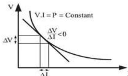
Figure 2. Negative impedance behavior of constant power load
