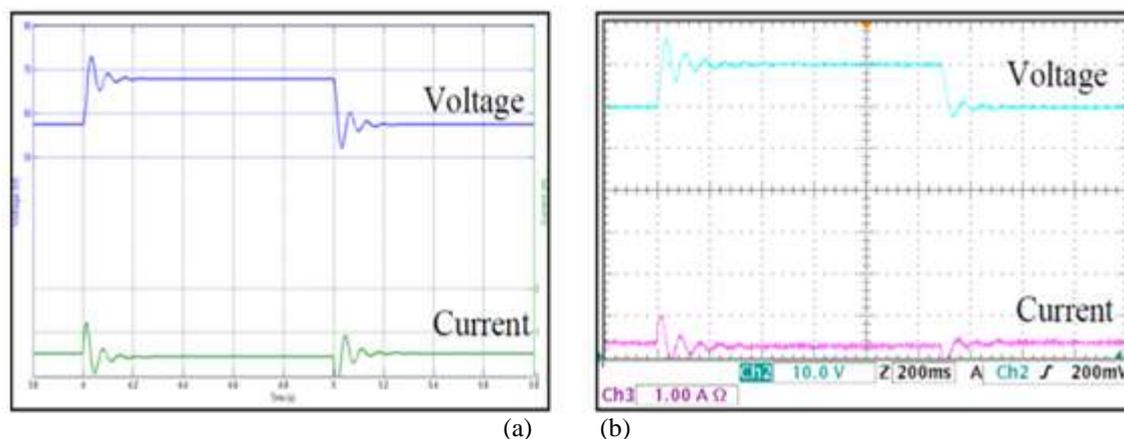
**Figure 15.** Plot of bus voltage and current with CPL= 30 W during input voltage transience without passive damper; (a) simulation (b) experiment
