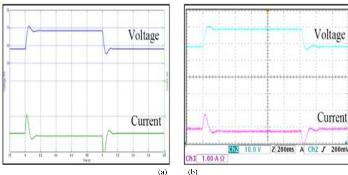
**Figure 17.** Plot of bus voltage and current with CPL= 60 W during input voltage transience with passive damper; (a) simulation (b) experiment
