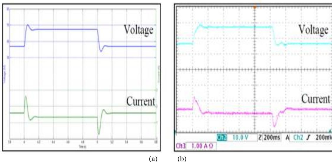
**Figure 16.** Plot of bus voltage and current with CPL= 90 W during input voltage transience with passive damper; (a) simulation (b) experiment
