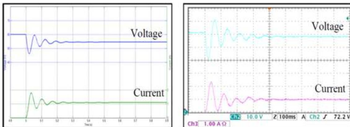
Figure 8. Plot of bus voltage and current with CPL= 60 W with CPL connection without passive damper; (a) simulation (b) experiment
